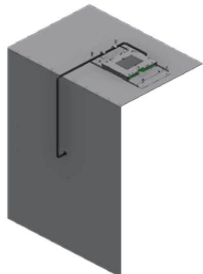
2m cable mounting – Display is mounted on fixture and processor is mounted top of car
