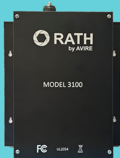
FIGURE 3: Image of the battery unit showing the mounting screw holes in the back
