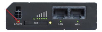
12. Wait 3 minutes for unit to fully boot. When fully booted, 4G LED should be illuminated along with at least 3 signal strength bars. If LEDs aren't as described, see troubleshooting section for corrective action.
