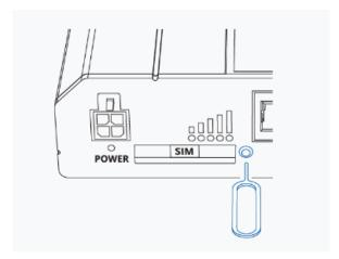
2. Pull out the SIM card holder and insert the SIM card using the provided SIM card adaptors if necessary.
