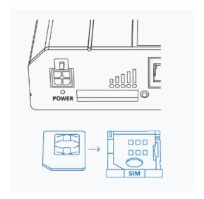
3. Slide the SIM card holder back into the cellular modem.
