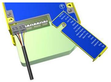
The following connections are required to the 20 way terminal block at the top of the Memcom unit...
