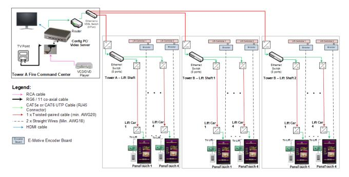
Note 1: The maximum length of the LAN cable (point-to-point inclusive of patch cable) is about 90m-100m. If length information is unclear, it is recommended a repeater or switch is installed. E-Motive supports Media-link solutions to extend the network beyond this.
