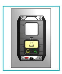
5. Insert tongue of SS plate in the groove at the top of the plastic housing
