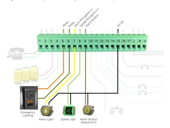
These connections are labelled on each of the wires connected to the accessory. Please note that when using the relay to switch on the emergency lighting for this accessory, you are not able to use the relay to switch on a siren when the alarm button is pushed. Both a COP accessory and siren can be wired into termainals 5 and 6 simultaneously, but the criteria to switch the relay has to be the same i.e. loss of power OR alarm button pressed.
