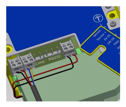
The following connections are required to the 20-way terminal block at the top of the Memcom unit.
