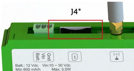
2. Connect the antenna on the MRL DCP to J2 and make sure it is completely screwed in.
