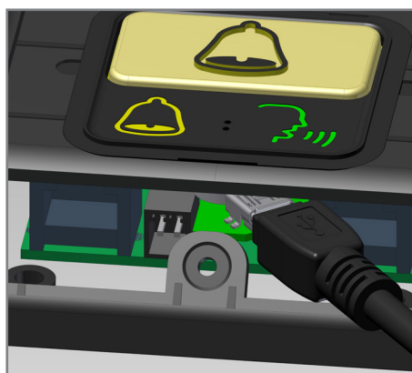
The entry port for C100 PT is between alarm button input and LVAS 2
